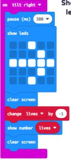
3. Repeat the code to detect the micro:bit tilting left or right
