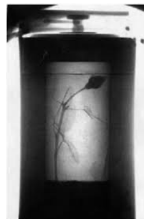
Image: Rose in a lead jar. Neutrons can pass through lead to allow us to see the rose inside.
