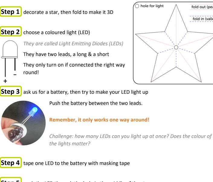
**Step 5** push the LED through the hole in the middle of the star.
