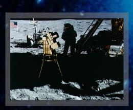
In 1972 the crew of Apollo 16 installed the first lunar astronomical observatory. The Far Ultraviolet Camera took pictures that would normally have been blocked by the Earth's atmosphere.
